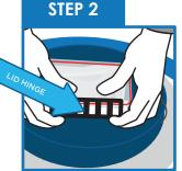
Unlatch data logger using thumbs to press against the black hinge.
