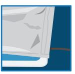
Place data logger back into the pouch and make sure to push the cable with the ferrite bead completely down into the bag. Push the cable into the far corner of the bag and reseal by pushing all the way across the zip lock seal.
