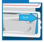
Fold the pouch in half and put the unit back into the protective box. Ensure that the cable is inserted into the slot to prevent cable pinching.
