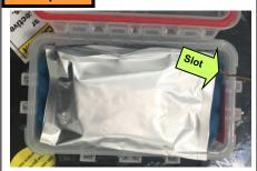
Fold the pouch in half and put the unit back into the protective box. Assure that the cable is inserted into the slot to prevent cable pinching
