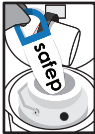
Retrieve and remove the Safepak®XL from the dewar.
