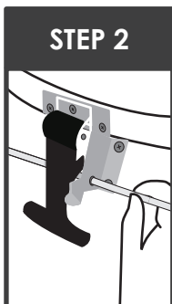
Insert zip-tie through one of the holes on the metal latch hardware.
