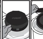
Open the hinged cap by pulling up on one of the two lift handles on the lid. With gloved hands, pull up on the circular handle in the center of the vapor plug to remove the vapor plug. Set the vapor plug aside.
