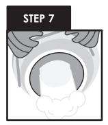
Pour off any excess liquid nitrogen by removing the lid and tipping the open end of the dry shipper toward the ground for two seconds.
