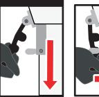
Latch handle on both sides by pulling the black handle down & then towards the shipper.
