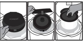
Open the hinged cap by pulling up on one of the two lift handles on the lid. With gloved hands, pull up on the circular handle in the center of the vapor plug to remove the vapor plug. Set the vapor plug aside.
