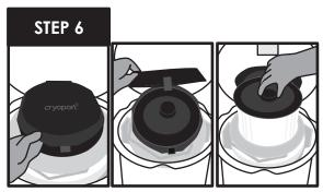
Open the hinged cap by pulling up on one of the two lift handles on the lid. With gloved hands, pull up on the circular handle in the center of the vapor plug to remove the vapor plug. Set the vapor plug aside.
