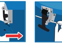
Insert zip-tie through one of the holes on the metal latch hardware.
