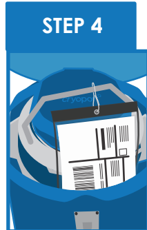
Remove the Leg 2 shipping pouch from the document protector attached to the dewar handle inside of the container.
