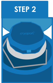
Close the hinged cap by pulling down on the lid.
