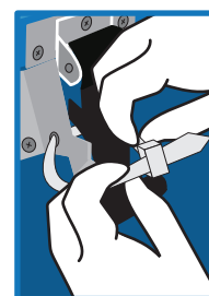
Insert zip-tie through the lid buckle and tighten.
