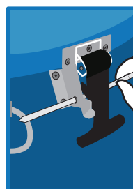
Thread end of zip-tie through the hole on the other side of the metal hardware.
