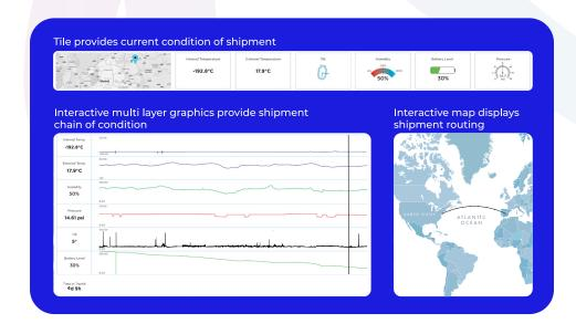
Figure 1: Cryoportal® 2 provides near real-time data about a shipment's internal temperature, external temperature, orientation/tilt, location, and other metrics.
