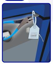
Prior to removal of the zip tie or serialized zip tie, record serialized number onto all pertinent documentation. Remove serialized zip tie with wire cutters.
