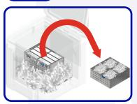
Remove Top Dry Ice Compartment with dry ice remaining inside. Properly dispose the dry ice from the Top Dry Ice Compartment.
