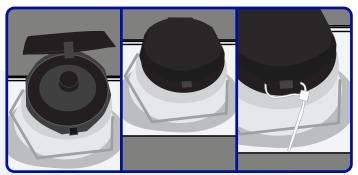
Reinsert the vapor plug. Close the hinged cap and secure it with a zip tie. Do not over tighten the zip tie as it will cause breakage.
