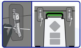
Insert the zip tie from left to right through each metal latch hole, wrap it around each latch, tighten it, and secure the lid.
