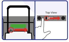
To unlock the metal handle, use one hand to slide the lever to the right and the other to lift or lower the handle.
