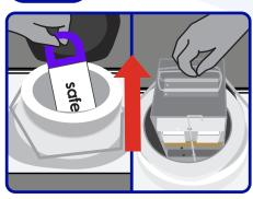
Slowly lift the packaged commodity out of the dewar by pulling upwards. Remove all secondary packaging.
