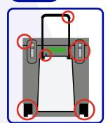
Once the shipping system arrives, check the enclosure and hardware for any damage that may have happened during transit.
