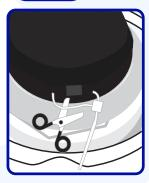
To access the dewar, open the lid and cut off the zip tie on the hinged cap with scissors.
