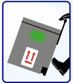
Place the shipping system on flat ground. See Step 4 to lift the metal handle with your hands, then place your foot at the bottom of the metal panel, tilt the shipper back, and use the integrated wheels to move it to the desired location.
