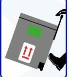
Place the shipping system on flat ground. See Step 4 to lift the metal handle with your hands, then place your foot at the bottom of the metal panel, tilt the shipping system back, and use the integrated wheels to move it to the desired location.
