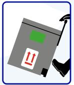
Place the shipping system on flat ground. See Step 4 to lift the metal handle with your hands, then place your foot at the bottom of the metal panel, tilt the shipping system back, and use the integrated wheels to move it to the desired location.
