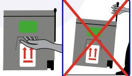
To unlock the metal handle, use one hand to slide the lever to the right and the other to lift or lower the handle.
