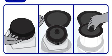
To remove the vapor plug, pull up on the circular handle located in the center. Place the vapor plug aside with the fleece lining facing up.
