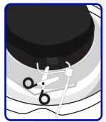
To access the dewar, open the lid and cut off the zip tie on the hinged cap with scissors.
