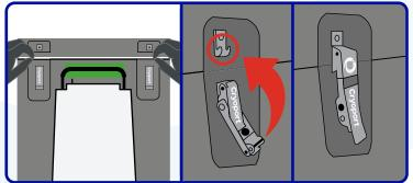
Close the lid and align it with the base. After aligning the enclosure, lift the latch handles and connect them to the hooks. Then, pull the latch handle down towards the enclosure until you hear a click to secure the latch. Complete this step for both latches.
