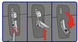
To unlock the latches, push the button located behind the latch handle and lift. To disconnect the top, pull the latch away from the hooks.
