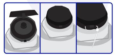
Reinsert the absorbent pad and the vapor plug. Close the hinged cap and secure it with a zip tie. Do not overtighten the zip tie as it will cause breakage.
