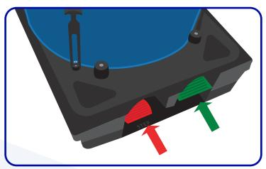
The Sliderite® pallet has two primary modes that are controlled by the pedals on either end of the pallet.
