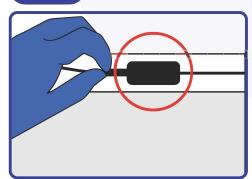
Remove the Smartpak™ thermocouple from the dedicated slot by pulling it out carefully.
