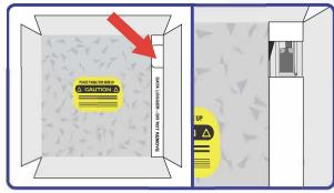
Find the data logger compartment and open the cover to access the Smartpak $^{\text{\tiny M}}$ .
