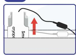
To remove the Smartpak™ in a secure manner, pull upward.
