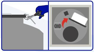
Use scissors to cut the zip tie located on the side of the vapor plug. Remove the vapor plug and set it aside with the Styrofoam facing up.
