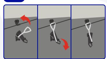
Lift the latch pin, connect it onto the hook, and push the handle down to latch both sides.
