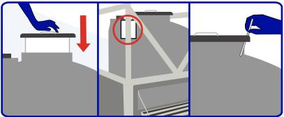
Reinsert the vapor plug and align it with the zip tie hole on the right side. Locate the zip tie in the clear travel pouch attached to the left side of the dewar. Insert the zip tie to secure the vapor plug to prevent tampering during transit. Do not overtighten the zip tie as it will cause breakage.
