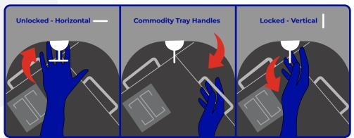
The shipping systems' commodity tray features four (4) compartments. To access the other compartments, pull the lock pin out towards you and turn clockwise until horizontal. Then use the handle in the middle of the compartments to turn the commodity tray and insert additional payload. To lock the commodity tray and prevent rotation, pull the lock pin out, turn it counterclockwise until it is in a vertical position, and you hear a click.
