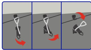
Locate the two (2) latches that hold the drop step in place. Then lift the latch handle and pull the latch pin away from the shipping system to unlatch both sides.
