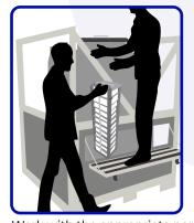
Work with the appropriate personnel to lift the payload and insert it into the shipping systems' commodity tray. To avoid temperature spikes, reinsert the vapor plug if there is a pause while loading the commodity tray.
