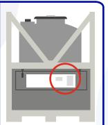
Locate the shipping envelope in the clear Leg 2 travel pouch attached to the left side of the dewar. Take out the labels/markings and place them on the drop step panel.
