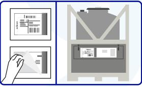
Pack the necessary documents into the Leg 2 envelope, with the air waybill on top. Then seal the envelope, remove the sticker backing, and place it on the drop step panel.
