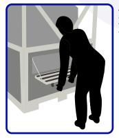
After the latching mechanisms are disengaged, carefully lower the integrated drop step with two (2) hands.
