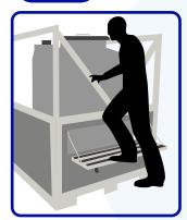
Once you release the step, hold onto the steel frame for support and prop your feet onto it to access the vapor plug. The max weight limit for the drop step is 300 lbs/136 kg.
