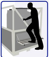
Hold onto the steel frame for support as you use the drop step to get down.
