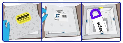
Remove the cooler lid and Phase Change Panel (PCP) to access the specimen chamber and unload your commodity.
