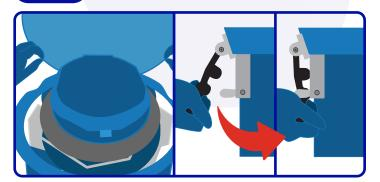
Close the lid and push the black rubber latch down towards the shipping system and connect it to the metal hardware. Complete this step for both latches.
