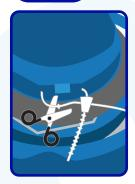
To access the dewar, open the lid and cut off the zip tie on the hinged cap with scissors.
