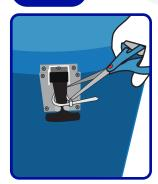
Use scissors to remove zip ties from both rubber latches.
