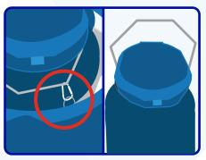
Disconnect the dewar from the enclosure by unlatching the carabiner behind the dewar. Remove the dewar by using the metal handle.
