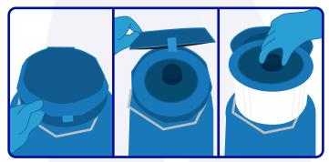
Open the hinged cap and pull up on the circular handle in the center to remove the vapor plug. Set the vapor plug aside, with fleece lining facing up.
