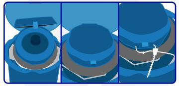
Reinsert the absorbent ring and vapor plug. Close the hinged cap by pulling down on the lid. Secure the hinged cap with a zip tie.
