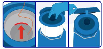
Slowly pour Liquid Nitrogen into the opening. Fill the dewar up to the bottom of the neck tube. Reinsert the vapor plug. Close the hinged cap by pulling down on the lid. Let the dewar stabilize in a static position for at least 60 minutes.
