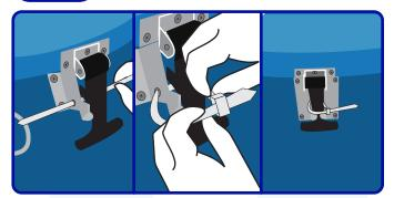
Insert the zip tie through each metal latch hole, wrap it around each latch, tighten it, and secure the lid. Do not over tighten the zip tie as it will cause breakage.
