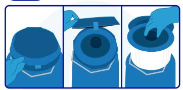
Once the dewar has stabilized, open the hinged cap and pull up on the circular handle in the center to remove the vapor plug. Set the vapor plug aside, with fleece lining face up.
