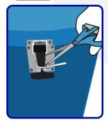
Use scissors to remove zip ties from both rubber latches.
