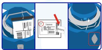
Locate the shipping envelope in the clear pouch on the dewar handle. Take out the label/marking and place it on the metal panel.
