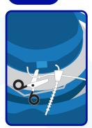
To access the dewar, open the lid and cut off the zip tie on the hinged cap with scissors.
