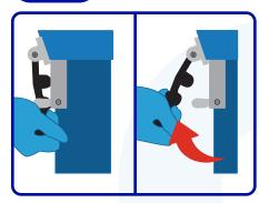
Unlatch both sides by disconnecting the black rubber handle from the bottom and pull the latch up and away from the shipping system.
