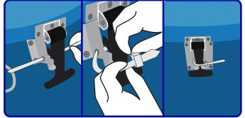
Insert the zip tie through each metal latch hole, wrap it around each latch, tighten it, and secure the lid. Do not over tighten the zip tie as it will cause breakage.
