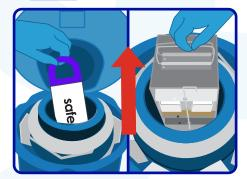
Slowly lift the packaged commodity out of the dewar by pulling upwards. Remove all secondary packaging.
