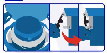
Close the lid and push the black rubber latch down towards the shipping system and connect it to the metal hardware. Complete this step for both latches.
