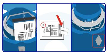
Locate the clear Leg 3 travel pouch attached to the dewar handle inside the enclosure. Remove the EMPTY label and place it.
