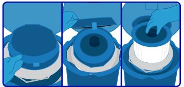
Open the hinged cap and pull up on the circular handle in the center to remove the vapor plug. Set the vapor plug aside, with fleece lining facing up.
