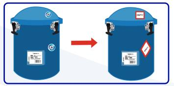
Place the other two (2) EMPTY labels over the BioServices labels on the enclosure and metal panel.
