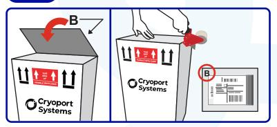
Close and seal the top of the box with packaging tape ensuring that Flap "B" is visible on the outside of the shipping system. The sealed envelope should be placed in the designated area on Flap
