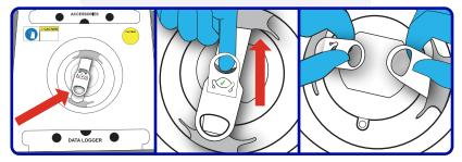
Locate the retention band featured above the vapor plug. Pull the small circular handle upward to release the retention band's locking tab. Then unlatch and separate the straps.
