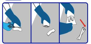
Use scissors to cut off the end of the Safepak® bag. Remove the contents and discard the bag. Reinsert the vapor plug and gently push it down into place.
