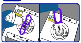
Remove the vapor plug and set it aside with the fleece lining facing up. Carefully lift the packaged commodity out of the shipping system and place it on a flat surface.
