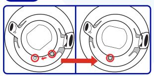
Ensure the tab on the vapor plug aligns with the gray tab on the dewar.
