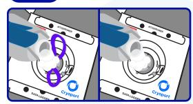
NOTE: Avoid spilling LN2 on the data logger.
