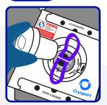
Reinsert the vapor plug. Let the shipping system stabilize in static position for at least 30 minutes. Make sure the Safepak® straps are left outside of the shipping system.
