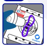
Carefully remove the vapor plug and set it aside with the fleece lining facing up. If using a Safepak® Bag, ensure the purple Safepak® straps stay outside of the dewar at all times.
