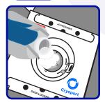
Slowly pour liquid nitrogen into the opening. (Cryoport Client Care will provide information on the amount of LN2 to use for your specific use case).
