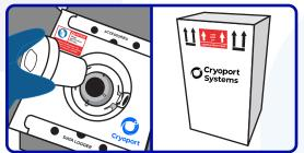
Reinsert the vapor plug and let the shipping system stabilize in a static position for at least 60 minutes.
