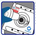
Once the shipping system has stabilized, remove the vapor plug and set it aside with the fleece lining face up.
