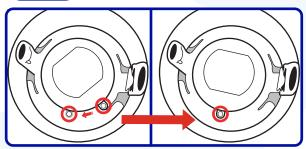
Reinsert the vapor plug. Ensure the tab on the vapor plug aligns with the gray tab on the dewar.
