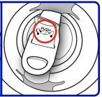
Place the "PUSH" tab behind the green check mark tab. The green check mark should be visible when secured.
