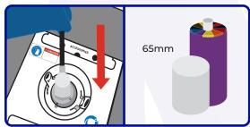
When using a 65 mm goblet (Daisy Goblet), place it onto the lifter and lower the commodity in the dewar.
