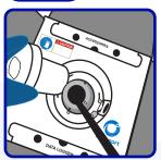
Reinsert the vapor plug and ensure that the black strap of the lifter is left outside of the vapor plug.
