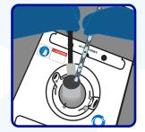
If the commodity is loaded in a goblet or vial on a cane, pull the black strap up to expose the top of the goblet and remove the cane.
