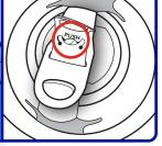
Place the "PUSH" tab behind the green check mark tab. The green check mark should be visible when secured.
