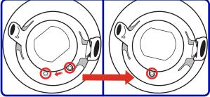
Ensure the tab on the vapor plug aligns with the gray tab on the dewar.
