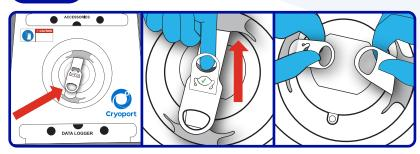
Locate the retention band featured above the vapor plug. Pull the small circular handle upward to release the retention band's locking tab. Then unlatch and separate the straps.
