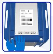
The lid must be opened one side at a time. Using one hand, press down on the lid while simultaneously pressing the latch release button. Pressing down on the lid will reduce resistance on the button and easily allow the latch to release.
