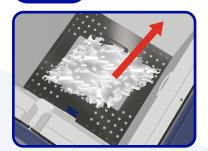
Remove and dispose any leftover dry ice in the Bottom Dry Ice Compartment.
