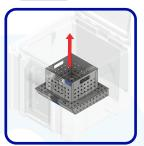
Remove the Payload Carrier to gain access to the Bottom Dry Ice Compartment.
