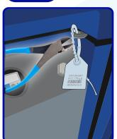
If a serialized zip tie is present, record serialized number onto all pertinent documentation prior to removal. Use wire cutters to remove serialized zip tie.
