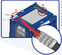
(A) Cut the straps if needed, and provide enough slack for the metal sealers.
