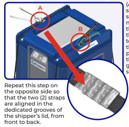
(A) Provide enough slack for the metal sealer, cut the strap if needed, then crimp the metal sealer onto the strap. (B) Use the tensioner to tighten the strap while positioning it within the designated grooves along the shipper's lid.
