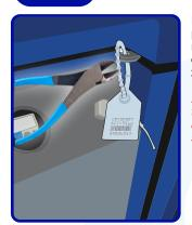
If a blue serialized zip tie is included, prior to its removal, record serialized number onto all pertinent documentation. Remove serialized zip tie with wire cutters.
