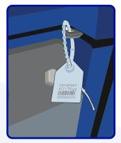
Add a zip tie (optional serialized zip tie ACC-9160) on the outside of the enclosure to secure the shipper. Record serialized number onto all pertinent documentation.
