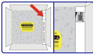
Find the data logger compartment and open the cover to access the Smartpak II®.
