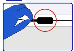
Remove the Smartpak II<sup>®</sup> thermocouple from the dedicated slot by pulling it out carefully.
