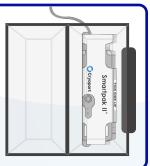
Locate the clear case to the left of the vapor plug to access the Smartpak II®. To open the case, release the black latch.
