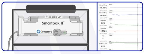
To manually upload the Smartpak II® data, tap and release the button featured next to the Cryoport logo. If the network LED light doesn't turn on after 5 seconds, tap and release the button again and repeat until you see a green light. After 5 minutes, refresh your Live View® link to see the stored data.
