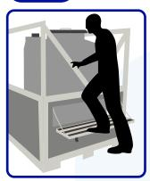
Hold onto the steel frame for support as you use the drop step to get down. Once your feet are on the ground, lift the drop step to reengage the latches on each side.
